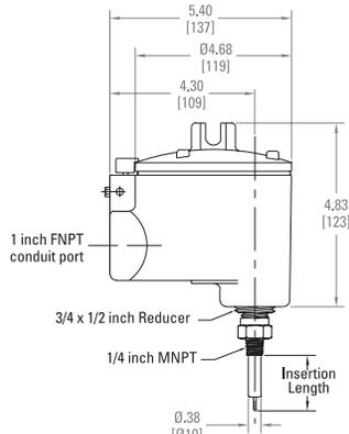
**With 316L Stainless Steel, All Welded Sensor**
